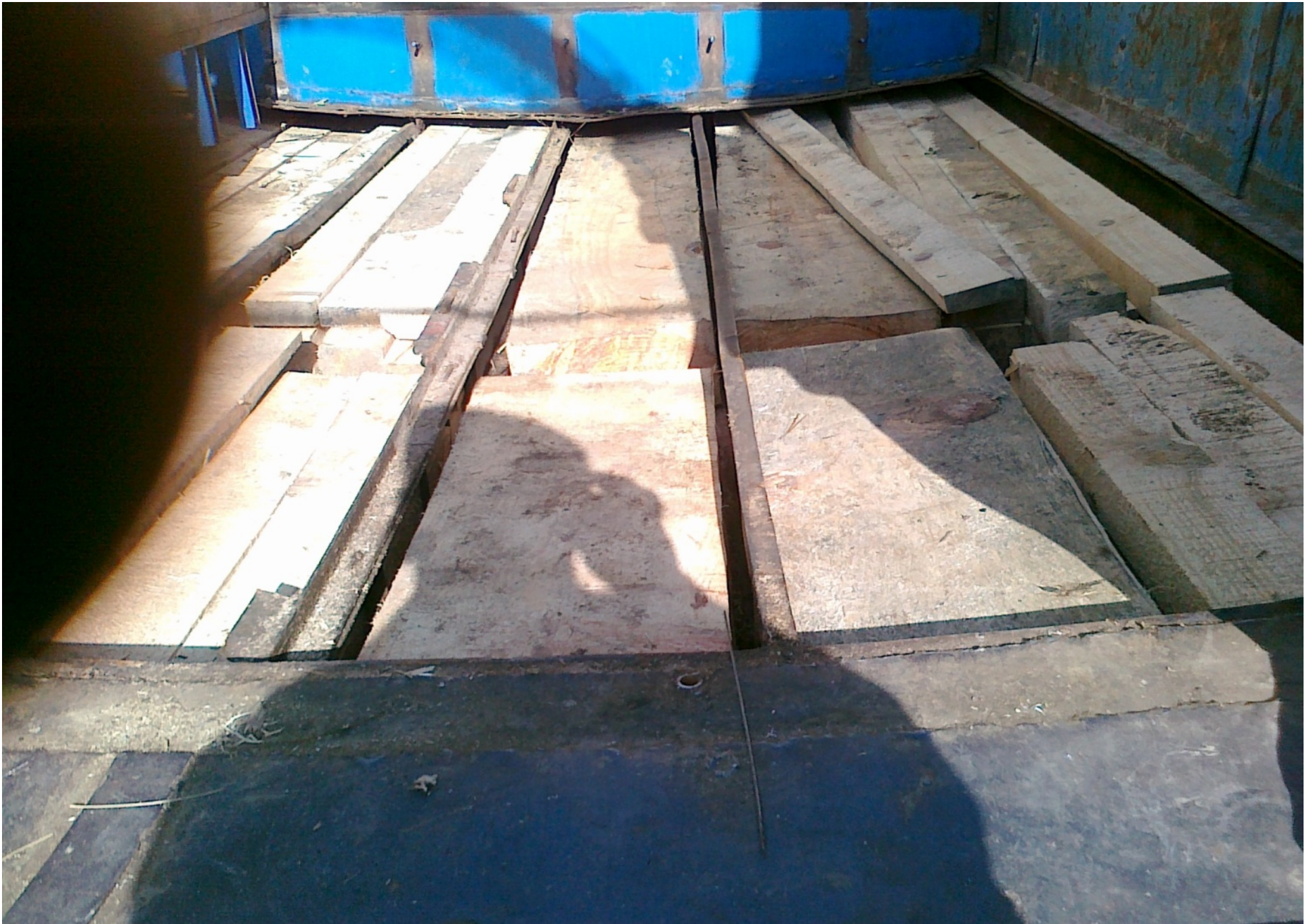
Truck floor specially fabricated for timber smuggling
